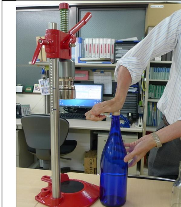
Apply the KT+KS cap to the bottle. Push-in the cap vertically and firmly until the end.
