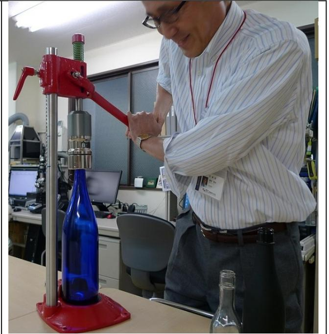
Press the handle underneath completely. Capping completed. Check the KT is firmly cramped, and does not turn easily.
