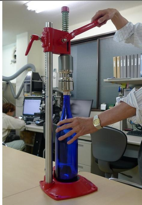
Place the bottle on the capper plate. Please remind, centering of crimping head and bottle.
