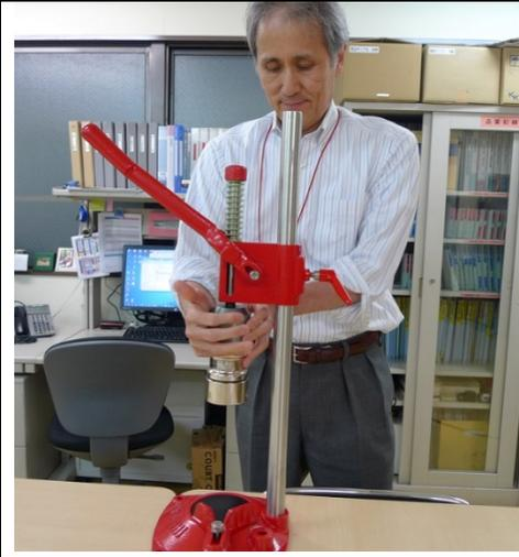
2. Insert the crimping head into the thread of capper.
