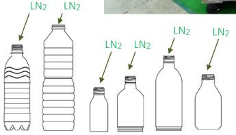
Designed for Bottle-Cans & PET bottles as illustrated on the left. Suitable for trial filling and small scale production of Bottle-Can products with positive pressure inside and experimental filling into lighter / thinner PET bottles.
