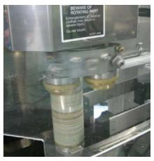
Seaming Head Assembly of BRX, composed of a 1st roller and a 2nd roller. (Closing head for Bottle Can's screw caps can be equipped.)
