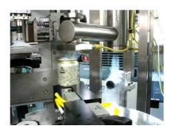
Recommendable LN2 Dosing Unit of VBC. Easily installed only connecting LN2 bin and its dosing head (photo above & right) with a special flexible vacuum hose. Operation through control unit (photo left) is also quite simple. (Other dosing heads can be used. The maximum head diameter is 300mm.)
