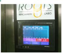
Filling process is controlled by PLC, checking the pressures of products and gas with sensors. Each parameter can be modified through its touch panel. Of course, special programs (displaying the variation of in-can pressure, gas exchanging before filling, etc) are available by request.
