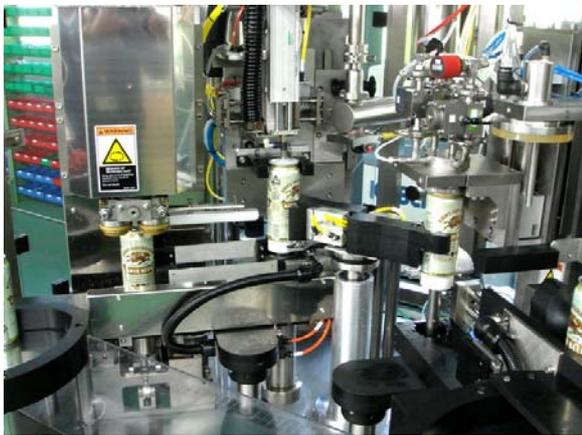
Photo of stations (right-in/left-out model): Air Rinsing (right end), Filling, Lid Feeding & Undercover Gassing, Seaming (left end)
