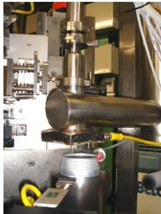
A filled can is gripped and quickly transferred under a LN2 dosing unit by a special swing arm. (Photo: the moment of LN2 dosing)
