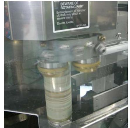
Seaming Head Assembly of BRX, composed of a 1<sup>st</sup> roller and a 2<sup>nd</sup> roller. (Closing head for Bottle Can's screw caps can be equipped.)
