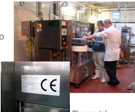
The special model capable to fill 7 types of can, exported to Europe with optional CE marking.
