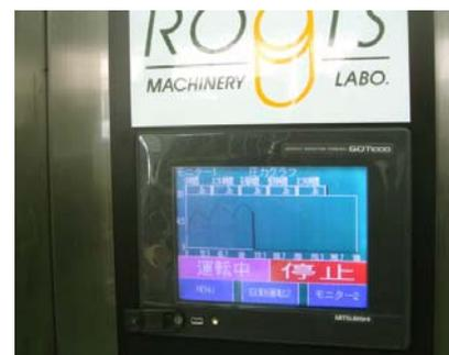
Filling process is controlled by PLC, checking the pressures of products and gas with sensors. Each parameter can be modified through its touch panel. Of course, special programs (displaying the variation of in-can pressure, gas exchanging before filling, etc) are available by request.
