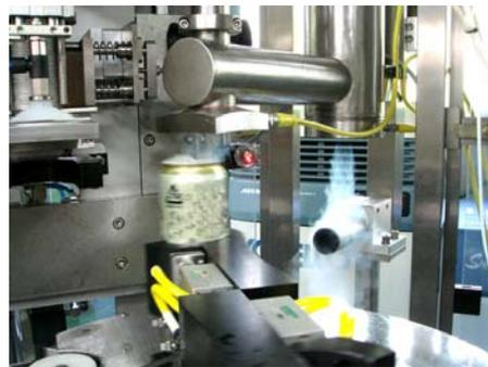
Recommendable LN2 Dosing Unit of VBC. Easily installed only connecting LN2 bin and its dosing head (photo above & right) with a special flexible vacuum hose. Operation through control unit (photo left) is also quite simple. (Other dosing heads can be used. The maximum head diameter is 300mm.)
