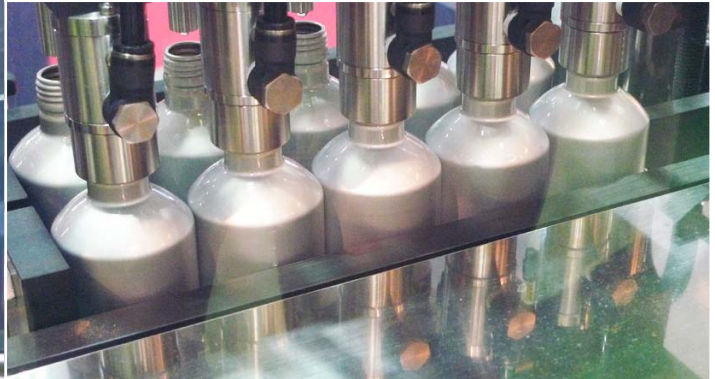
Air-rinsing and then filling 5 bottles simultaneously. The filling nozzles don't touch bottle mouth.
