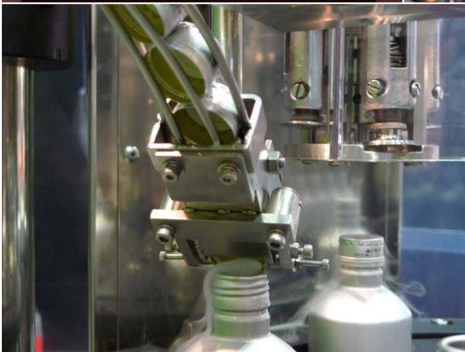
Zalkin capping head as standard setting for Bottle-Cans. (Other heads can be set by request)
